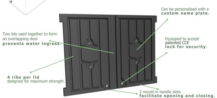
Can be used as **doors for Skips, Rolonoff containers, bottom opening containers** and closed containers.
